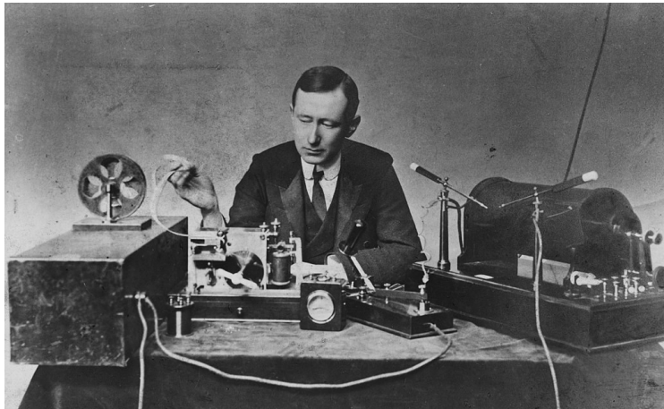
Marconi, 1901, with his early spark transmitter (on his left) and coherer receiver (his right), which recorded the Morse code symbols with an ink line on paper tape
