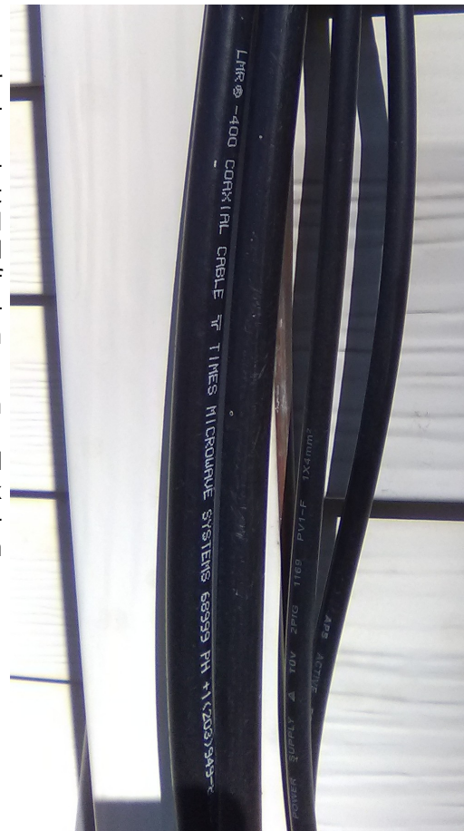
My humble bundle: LMR-400 for VHF, LMR-400 for HF, MC4 for solar, all spread out for a photo op, plus a 4 AWG ground wire in back
