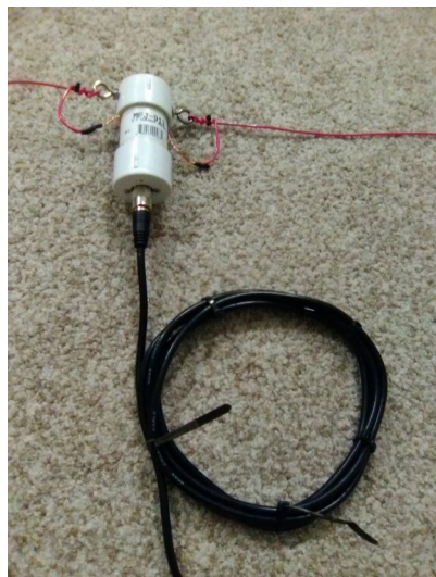
RF choke zip tie-secured
