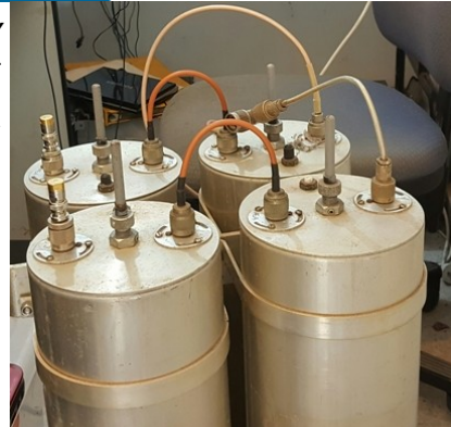
repeater cavity filters
