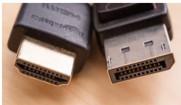
HDMI (left) and DisplayPort (right)
