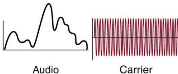
We still need to convey the same two pieces of information: loudness and pitch. Once again, we start with the audio (your voice) and a carrier (radio frequency) signal. An FM transmitter contains circuitry that not only changes the carrier frequency, but changes it at a certain rate, which is the frequency of your speech.
