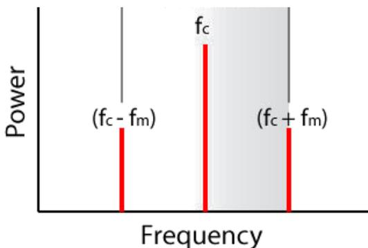
So, AM is the re-shaping of a carrier amplitude by your voice before sending it out, and FM is the continual modifying of a carrier frequency by your voice.
