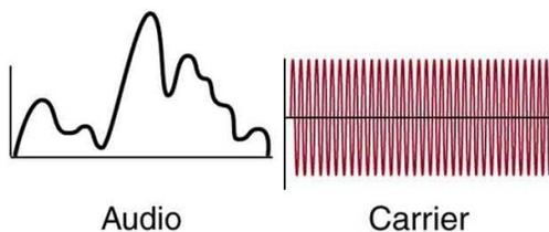
carrier frequency. An AM transmitter contains simple circuitry that can shape the carrier so that, instead of being a constant level, its peaks and valleys (loudness) and sharpness (pitch), match those of your voice. What we end up with is a radio-frequency signal (carrier) that has been changed (modulated) by your voice and can now be transmitted
