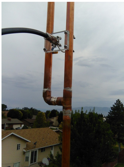
Finished J-pole, bottom end
