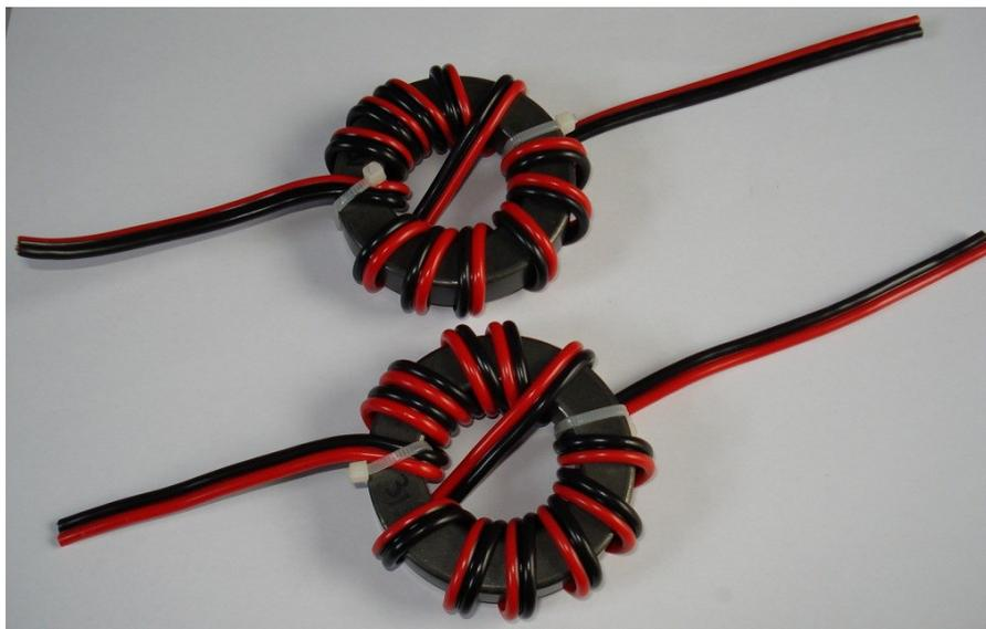
cross the pair over then under the diameter to wrap six more turns in the same direction, but on the other side of the pair. Zip-tie the two ends to secure them in place, leaving about six inches of wire pair on each end to work with, then strip all eight wire ends. (For reference, the *transceiver end* is on the left side in this photo, and the *antenna end* is on the right.)
