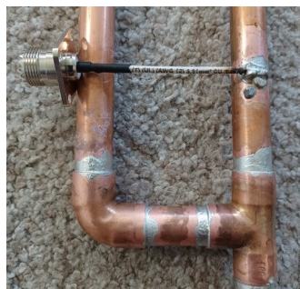
Solder the wire and bolt the connector
